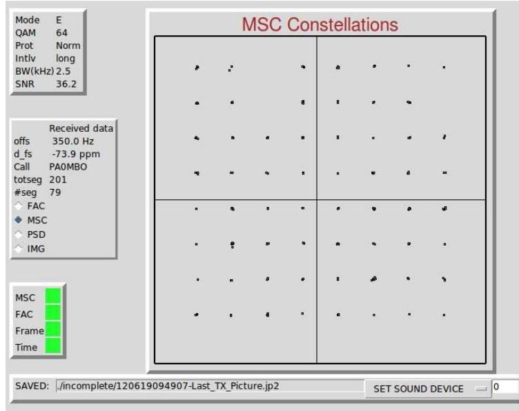
Figure 4: GUI showing MSC-constellation
