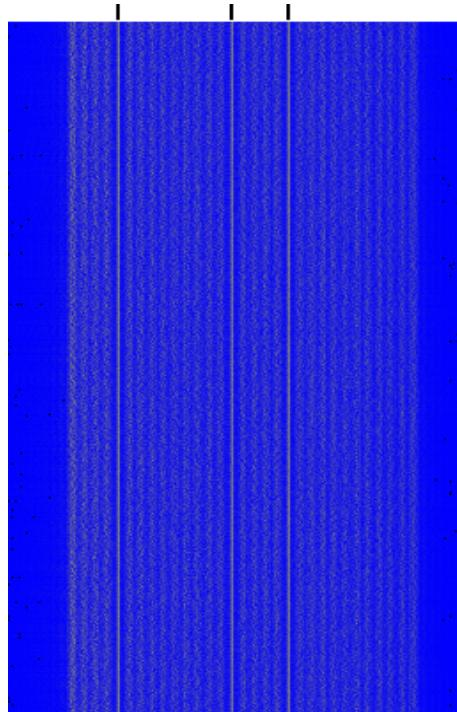
Figure 3: Waterfall window with DRM signal
